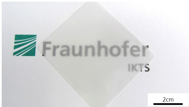
Tape casted and sintered solid electrolyte (100 \mu\text{m} thickness).
